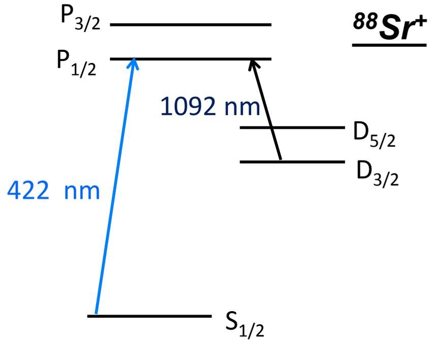
422 nm: Laser cooling/state detection
